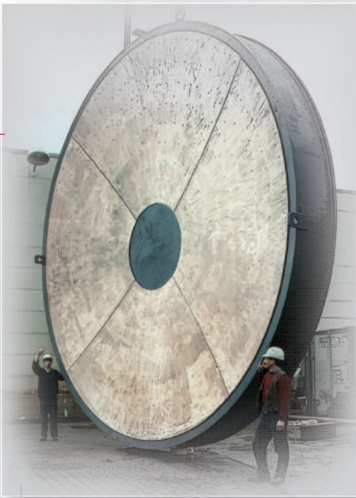
▶ BOTTOM ELECTRODE \varnothing 7.0 m
